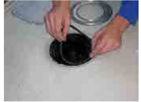
3. Remove lid cover, clean flange and insert the gasket
